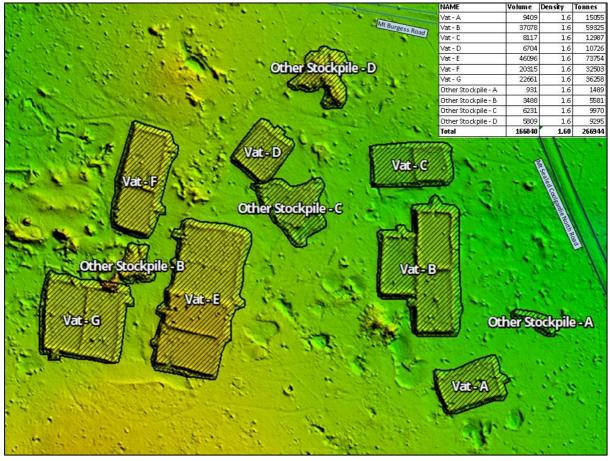
Figure 6: Plan view of shaded digital elevation map with the main historic Bonnie Vale Tails deposits labelled with summary table for tonnage. The inset table provides details of volumes calculated using high resolution survey.
