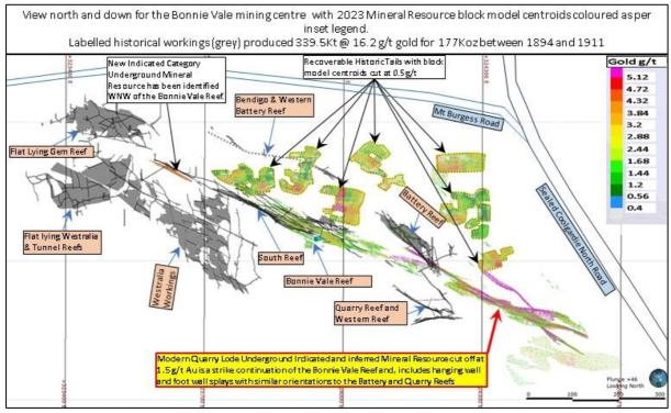
Figure 3: View north and down with partially transparent satellite imagery over 3D historic mine development (grey polygons) with labelled features and 2023 Bonnie Vale underground Mineral Resource block model centroids coloured for gold g/t as per inset legend.
