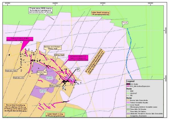
Figure 4: Plan view for the Bonnie Vale area with simplified geology showing the Bonnie Vale Granitoid intruding the core of an F3 anticline. The surface position of high-grade veins are marked by magenta polylines. The Bonnie Vale mineralised quartz veins are hosted within the Bonnie Vale Granodiorite
