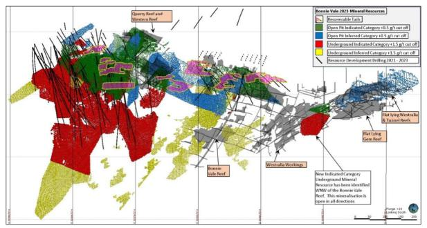
Figure 1: Oblique view looking down toward the south showing Bonnie Vale: Open Pit, Underground and Tails Mineral Resource block model centroids coloured as per inset legend. Drill traces (Black lines) for resource development infill drilling completed between 2021 and 2023 are also shown. Historic Bonnie Vale mine workings are labelled and represented by semi transparent grey polygons.
